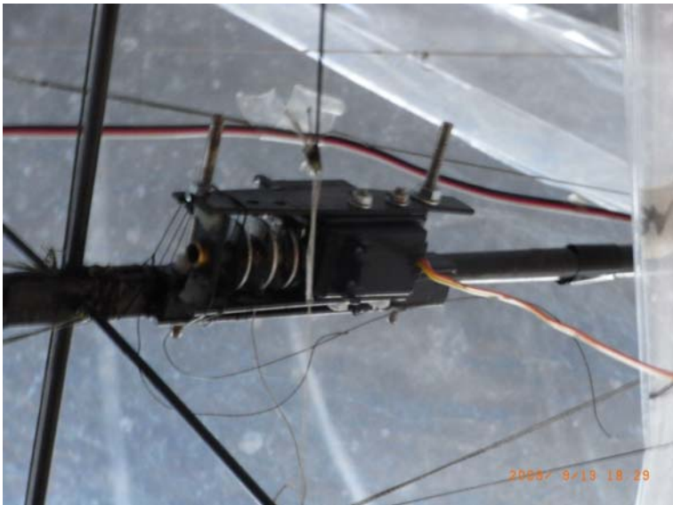
Futaba 3151 servo converted to winch, moving hinge 3 by pulling/releasing a small cable.
