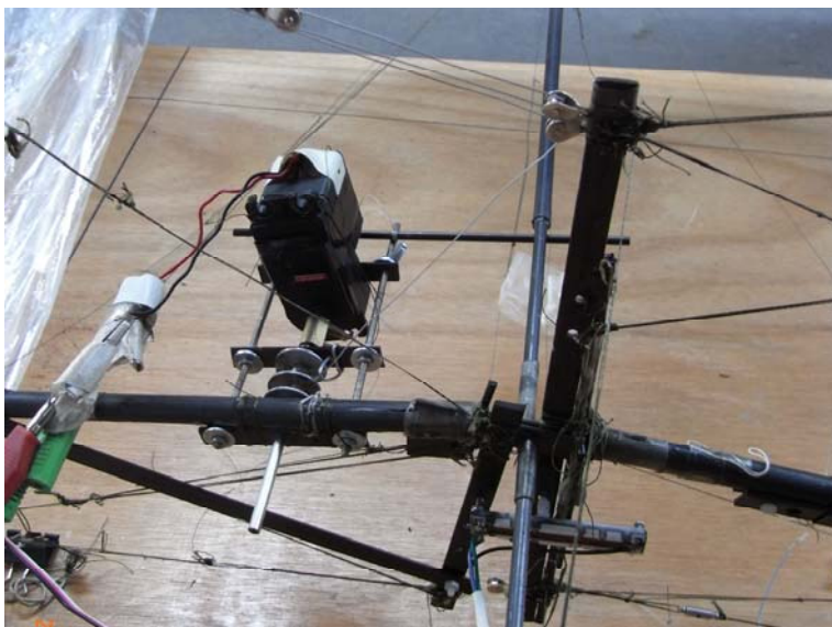
Vertical hinge, showing the Hytec servo with winch, the hinge itself, and the position sensor, a slide resistor, at the bottom of the picture.
